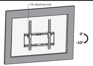
Loosen the adjusting knobs to tilt to desired angle then retighten them.
